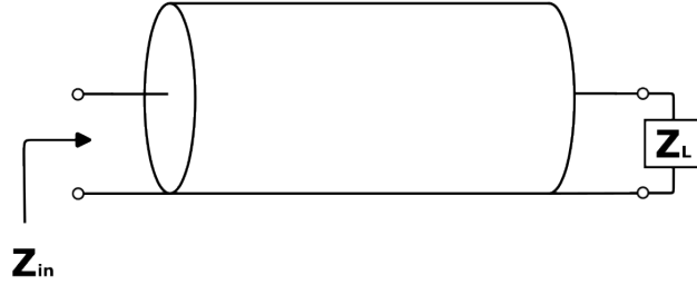
Figure 2.3: Transmission Line Input Impedance. We can connect a load Z_L to the transmission line, shown here schematically. This allows us to interact with the load over a long electrical distance, or we can interpret this as altering the electrical properties of the transmission line itself (understood by calculating the input impedance Z_{in} ).
